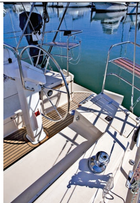
A lift-up section of coaming gives access to the stern boarding platform.
