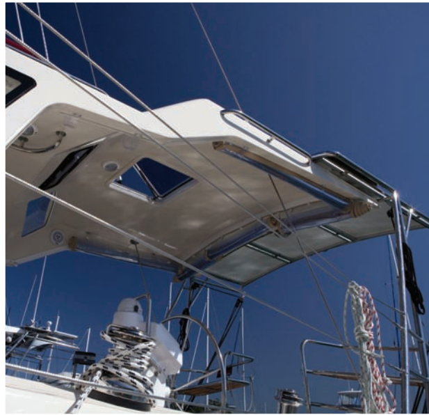
LEFT: A hard-top dodger-cum-bimini with clears gives the helmsman total protection when needed.
